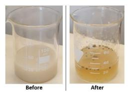
**The Solution:** We have implemented our SOA-AFA solution as a treatment agent based on batch treatment approach. As it shown below, our reagent is an efficient reagent for this type of wastewater, with a **conversion of 99% for 1, 4-Dioxane and 95% for hydrocarbons after single treatment**.
